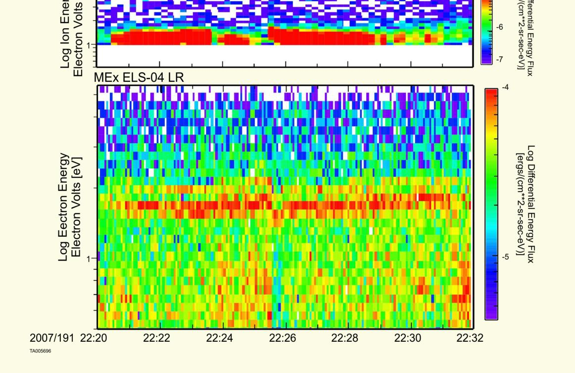
Figure 2. ASPERA-3 Electron and Increased Sensitivity Ion Spectrograms. Shown is data from 10 July 2007 in the Martian ionosphere. Sensitivity to low-energy ions has been increased so that they can be and are observed.
