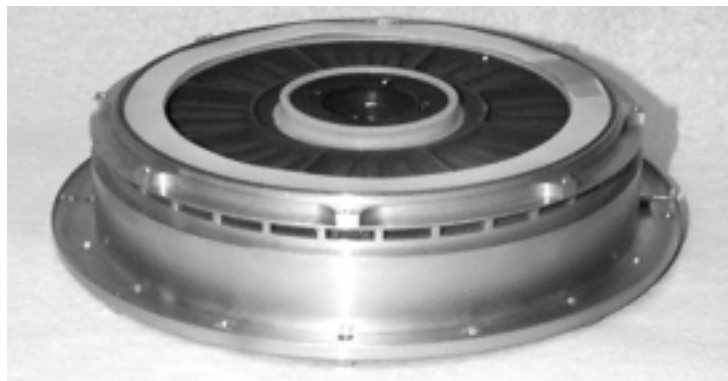
Figure 3.2.2. The low energy neutral particle imager for the ASPERA-C/Mars-96 experiment (spare unit).
